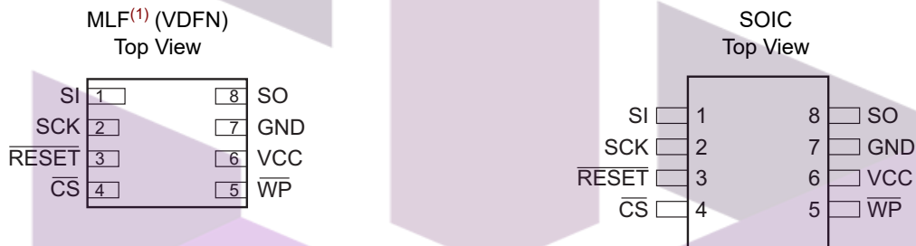
Figure 1-1. Pin configurations and pinouts.
